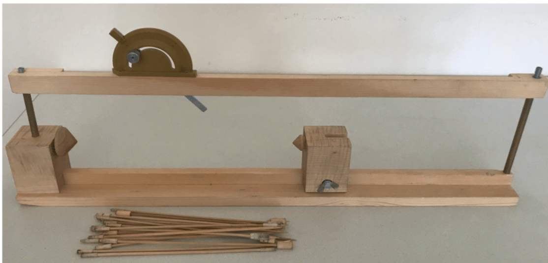
Fig. 5 Framework to hold joint horizontally, with padded sticks
